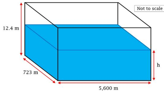
**Figure 1:** Diagram showing the structure and measurements of our model reservoir.
